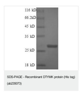
(Tris-Glycine gel) Discontinuous SDS-PAGE (reduced) analysis with 5% enrichment gel and 15% separation gel of ab235073.
