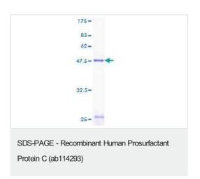
ab114293 analysed on a 12.5% SDS-PAGE gel stained with Coomassie Blue.
