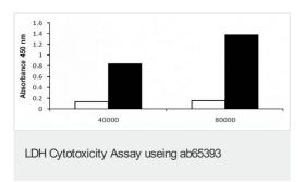
Jurkat T cells were cultured in 96-well plate in 100 µl of culture medium. LDH Assay was performed using 10µl of culture medium using the WST probe. Low control (white bar); High control (black bar).
