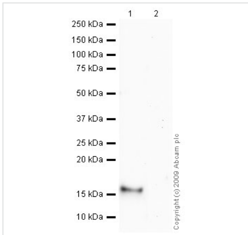
Western blot - Anti-Histone H3 (tri methyl K4) antibody [mAbcam1012] - ChIP Grade (ab1012)
