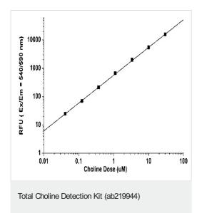
Typical Choline standard calibration curve. Choline dose response was measured on a 96 well solid black plate using a Gemini fluorescence microplate reader (Molecular Devices). As low as 40nM (4 picomole/well) of choline can be detected with 30 minutes incubation time (n=3).
