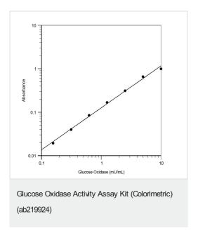
Glucose Oxidase Activity Assay Kit (Colorimetric) (ab219924). Typical glucose oxidase dose response curve. Absorbance was measured on a 96-well clear bottom plate using a SpectraMax microplate reader with path check on.
