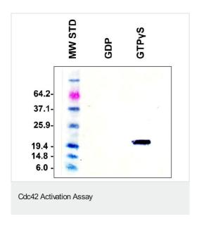
Lane 1, MW Standard. Lane 2, 293 cell lysate loaded with GDP and incubated with PAK PBD Agarose beads. Lane 3, 293 cell lysate loaded with GTP $\gamma$ S and incubated with PAK-1 PBD Agarose beads. Samples were immunoblotted with anti-Cdc42 antibody.
