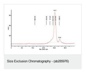
Size exclusion chromatography analysis of ab285976 (after removal of DTT, EDTA and glycerol) using a Supersex 200 HR 10/30 column at 0.5ml/min in 50 mM Tris and 0.25M NaCl, pH 7.5.
