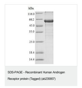
(Tris-Glycine gel) Discontinuous SDS-PAGE (reduced) analysis with 5% enrichment gel and 15% separation gel of ab235857.
