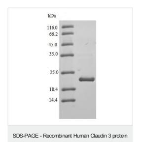
(Tris-Glycine gel) Discontinuous SDS-PAGE (reduced) analysis with 5% enrichment gel and 15% separation gel of ab235064.
