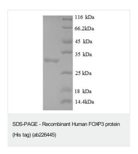
(Tris-Glycine gel) Discontinuous SDS-PAGE (reduced) analysis of ab226445 with 5% enrichment gel and 15% separation gel.
