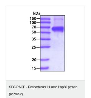
SDS-PAGE analysis of ab78792 at 3µg under reducing condition.
