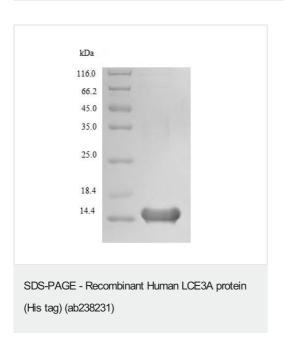
(Tris-Glycine gel) Discontinuous SDS-PAGE (reduced) with 5% enrichment gel and 15% separation gel analysis of ab238231.
