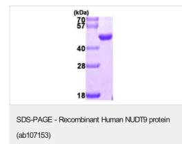
15% SDS-PAGE showing ab107153 (3μg). Note: Molecular weight on SDS-PAGE will appear higher.
