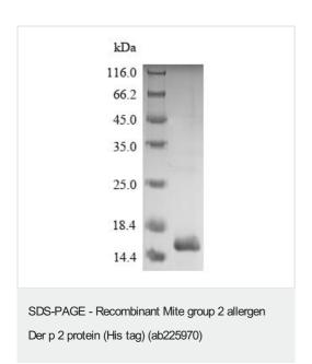
(Tris-Glycine gel) Discontinuous SDS-PAGE (reduced) analysis of ab225970 with 5% enrichment gel and 15% separation gel.
