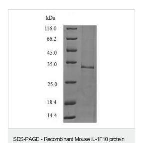
ab239445 analyzed by (Tris-Glycine gel) discontinuous SDS-PAGE (reduced) with 5% enrichment gel and 15% separation gel.
