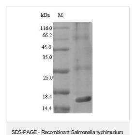
(Tris-Glycine gel) Discontinuous SDS-PAGE (reduced) with 5% enrichment gel and 15% separation gel analysis of ab235725.
