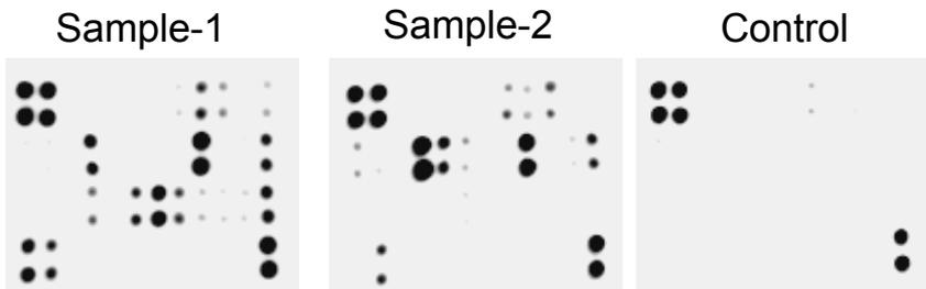
The preceding figure presents typical images obtained with Abcam Human Cytokine Antibody Array. These membranes were probed with conditioned media from two different cell lines. Membranes were exposed to film at RT for 1 min.
