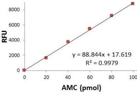
Figure 1. Typical AMC Standard calibration curve.
