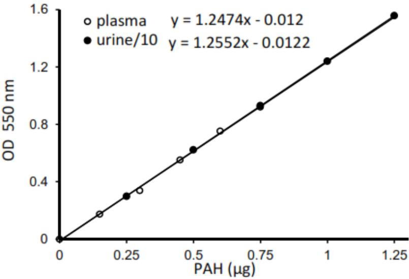
Figure 1. Typical PAH Standard calibration curve
