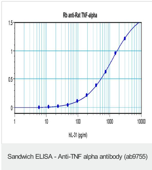
Sandwich ELISA of ab9755. This antigen affinity purified antibody, in conjunction with compatible secondary reagents, allows the detection of 0.2 - 0.4 ng/well of recombinant rTNF-alpha.
